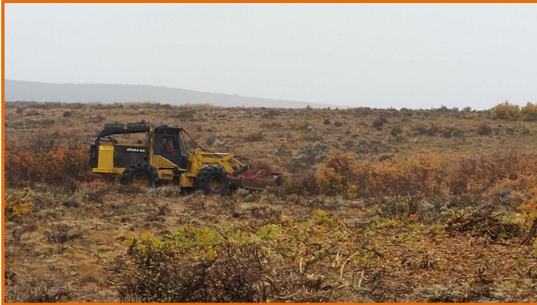
A machine called a Hydroaxe masticates oak brush in an effort to invigorate herbaceous and woody plants to improve habitat for big game and GUSG.
