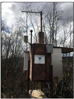
Photograph showing BLM automated stream gage instrument shelter and GOES satellite telemetry antenna, top center of photograph, at Birch Creek WSR River Mile 0.
