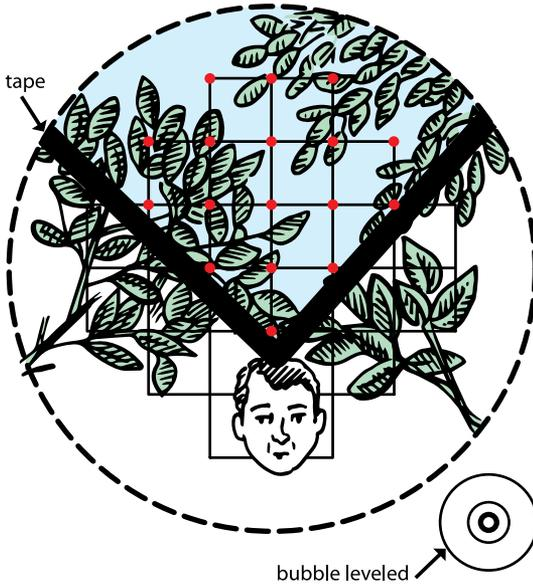
**Figure 16.** Modified densiometer. Count and record the number of grid intersection points within the V (0-17) that are covered by any form of vegetation or any object that creates shade, such as a canyon wall or bridge. In this example, the score would be recorded as 10 (USEPA 2009).
