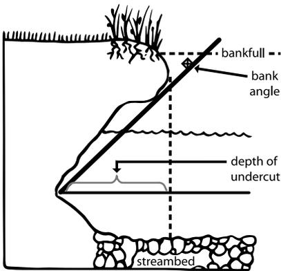
**Figure 30.** Measure undercut bank angle from the deepest point to the ceiling of the undercut; determine if the undercut has a qualifying depth ( $\geq 5$  cm) by lowering the depth rod until it is horizontal (Archer et al. 2015).
