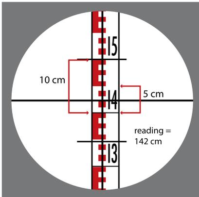
**Figure 26.** A stadia rod as viewed through the auto level. Stadia rods are broken up into 10-cm sections, denoted by the large number on the right. On this stadia rod, each cm is identified by alternating red and white blocks. The top and bottom of each block are equal to 1 cm. In this image, the measurement would be recorded as 142 cm.
