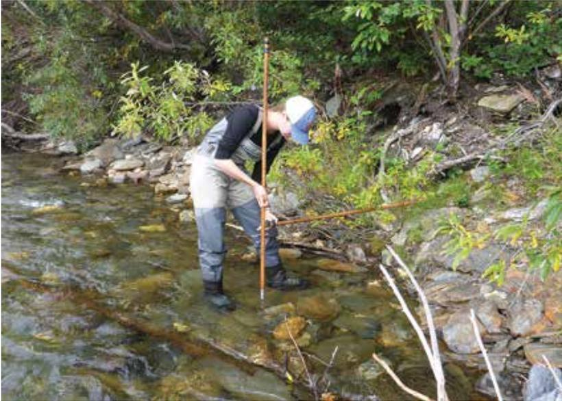
**Figure 4.** Example of how to use two depth rods to measure bankfull or bench height. For this transect, bankfull and bench height are at the same elevation. Note the position of the horizontal depth rod, which is at the same elevation of the flat, bench surface.
