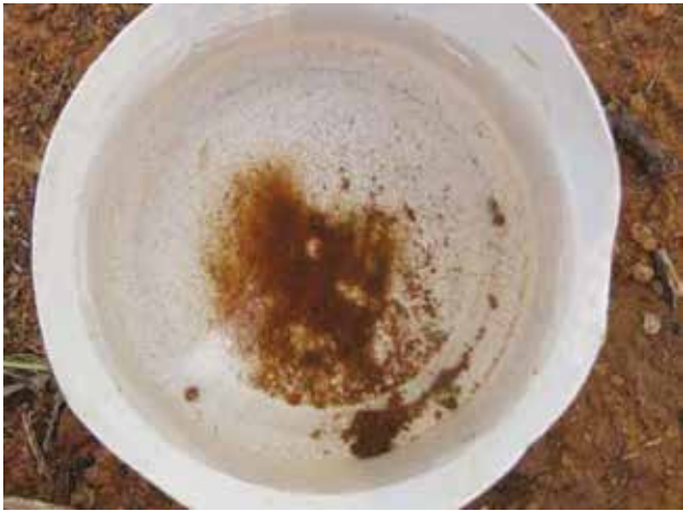
Figure A9.1. Soil sample that disintegrated when swirled.
