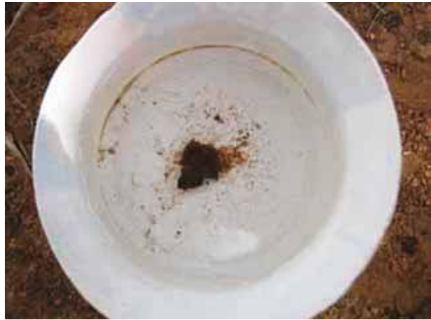
Figure A9.2. Soil sample that remained stable, even after swirling.
