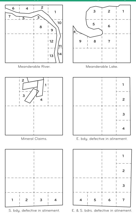
**Figure 3.** Examples of subdivision of sections by protraction and showing lots.
