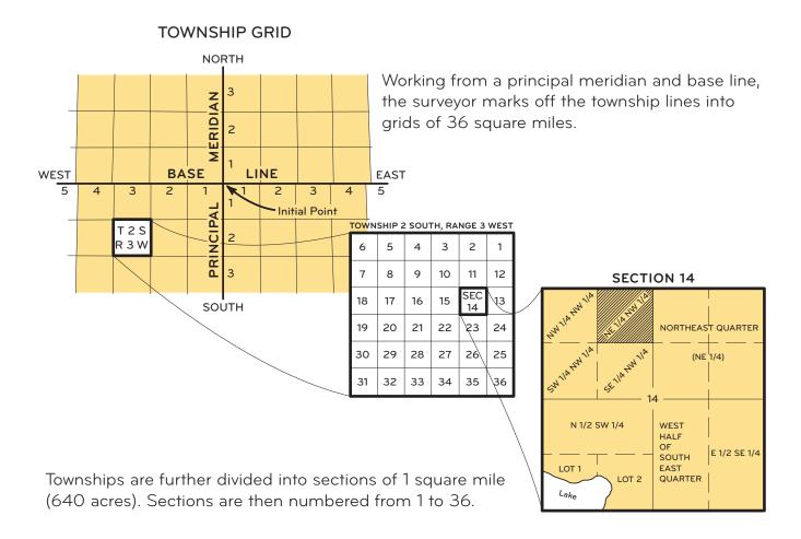
**Figure 2.** Example of township and range lines for the establishment of townships, section lines for the establishment of sections, and subdivision of section lines for the establishment of aliquot parts and lots of a section.
