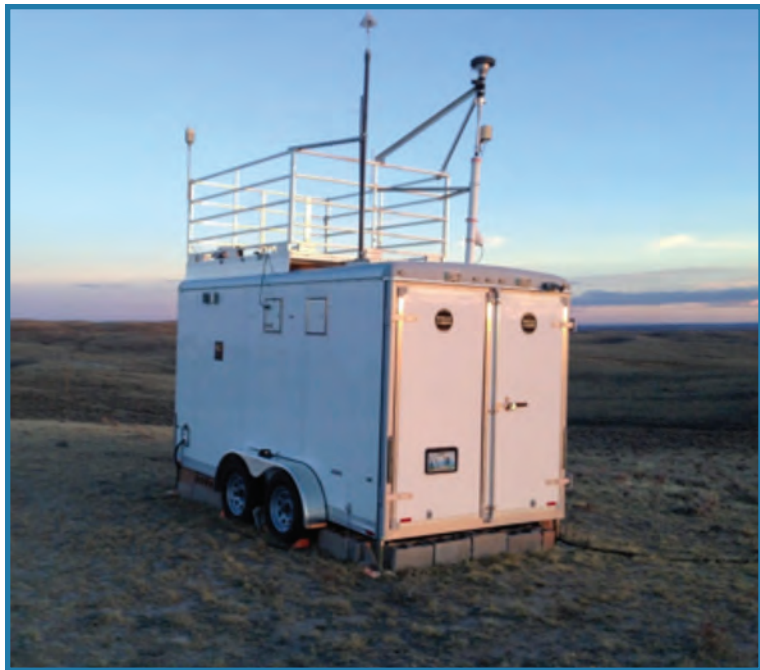
The University of Wyoming's mobile air quality laboratory at the Blizzard Heights site in Converse County, Wyoming.
