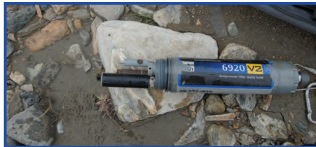
Automated multiparameter water quality meter used in the Fortymile Wild and Scenic River water quality study.
