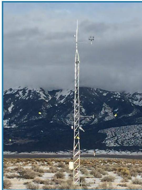
The 33-foot-tall meteorological tower at the wind erosion monitoring site in the San Luis Valley.
