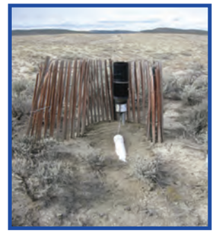
An upgraded rain gauge with a precipitation adaptor and waste antifreeze reservoir at Wolf Creek.
