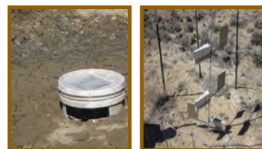
Dust and wind erosion monitoring equipment in Badger Wash.
