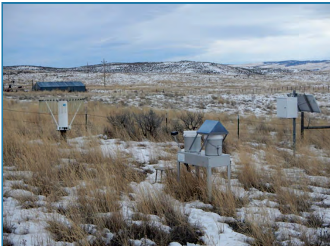
Equipment at the Sand Springs National Atmospheric Deposition Program site in the BLM Little Snake Field Office that is used to help sample precipitation chemistry and quantity in northwest Colorado.
