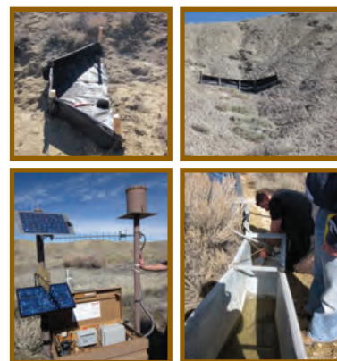
Silt fences constructed in western Colorado and hillslope erosion and climate and flow monitoring equipment.
