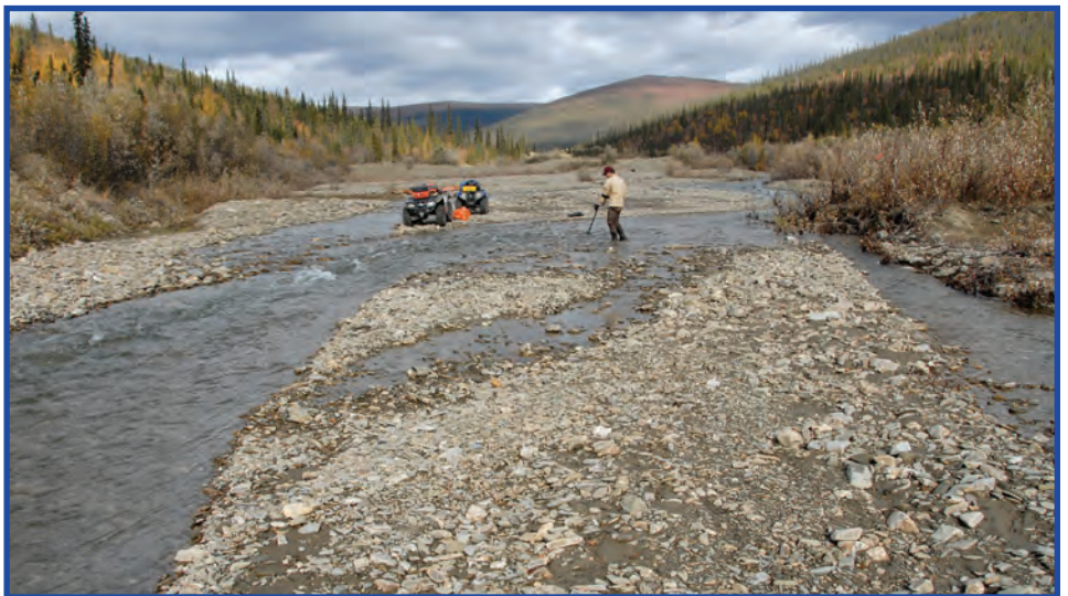
This view is upstream on a placer-mined tributary of Birch Creek and shows a BLM hydrologist measuring water quality in a highly active coarse gravel stream channel. High bedload sediment transport rates are common in highly disturbed, high-gradient placer-mined watersheds.
