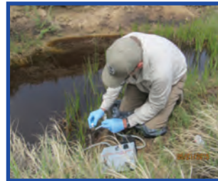
A White River Field Office employee uses a peristaltic pump to collect water samples from a spring above Rangely, located in an abandoned oil well.
