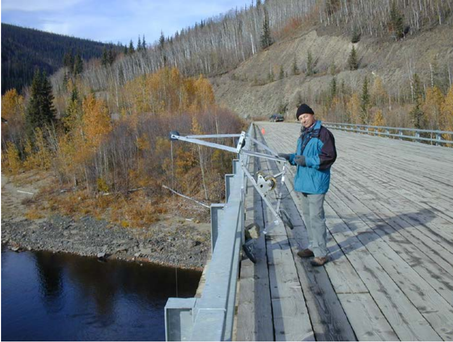
Fig. 2. Where the river was too deep to wade, such as the Fortymile River at the Taylor Highway Bridge, a flow meter and sounding weight were suspended by a cable and reel system to survey the river.
