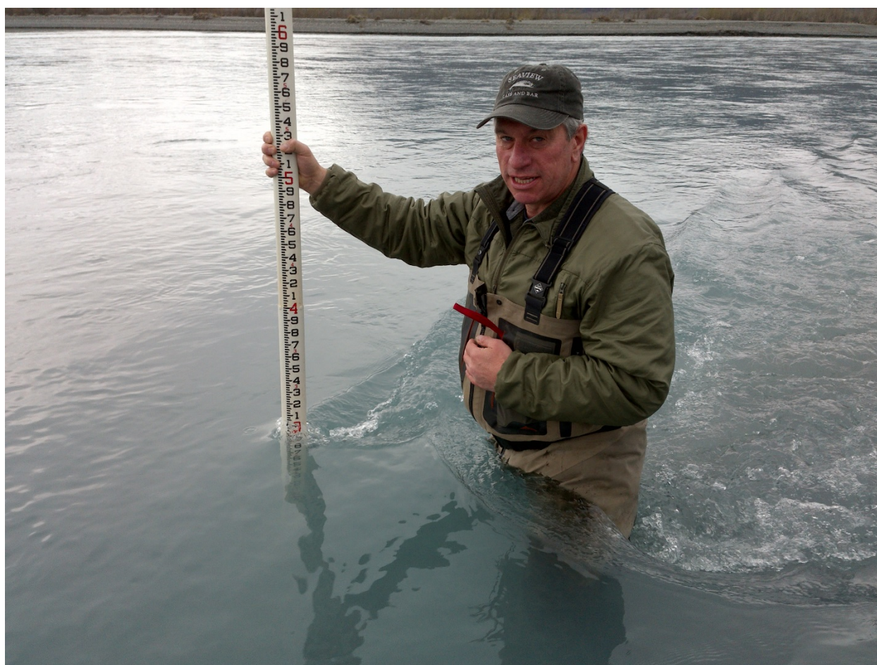
Figure 3: Merlyn Shelske, recording the depth of the Knik River at a location near the western township line of T. 16 N., R. 4 E., SM. The depth noted on the survey rod shows approximately 3 feet.
