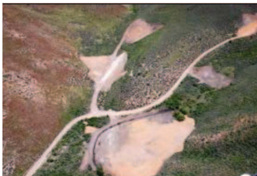
Rip Creek diversion and reclaimed ponds: In the middle foreground the extensive armored creek channel diversion is visible, moving flowing water around the tailings to avoid contact with them.
