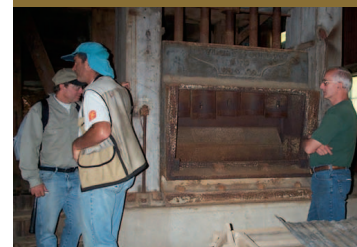
Inside view shows mill equipment including the stamp battery where the ore was pulverized and mixed with water to form a pulp still intact.
