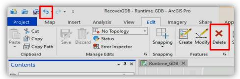
The Activated Delete Tool and the Undo Tool in ArcGIS Pro
