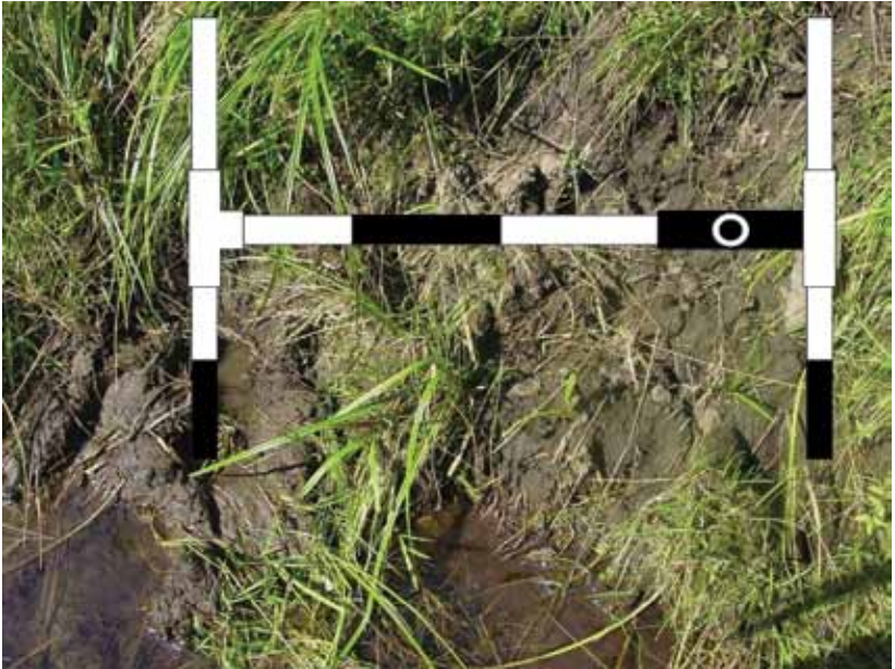
Figure E13. Trampling by large herbivores has caused obvious “slumping.” The slump is greater than one-fourth of the plot length and is recorded (S).
