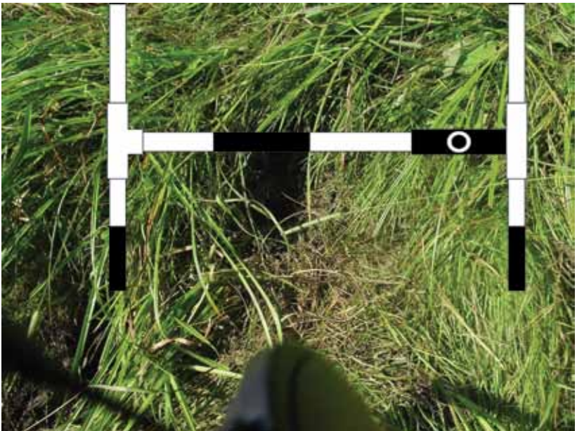
Figure E14. There is a hoofprint in the bank, but no slump or slough is associated with the hoofprint; therefore, there is no indicator of instability so covered (C) and absent (A) are recorded.
