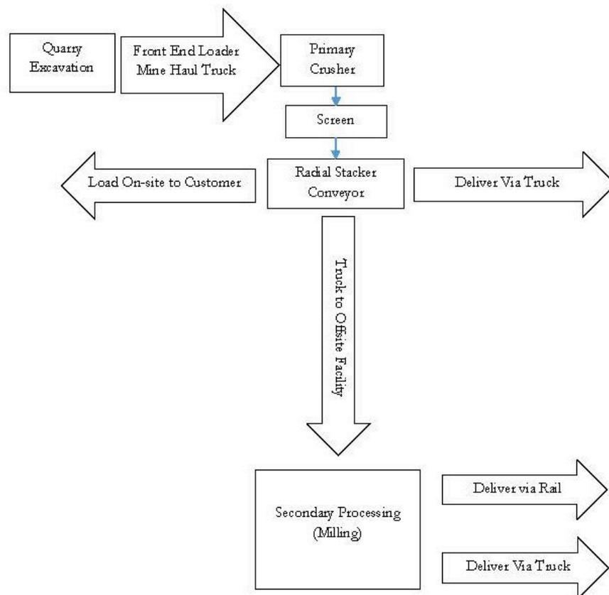
HQP would be loaded onto trucks in the mine area, trucked to the scales located on KMC's adjacent privately owned lands where they would be weighed and sent to market. Truck transport would be used for delivery to customers within an approximately 350-mile radius of the Site and rail transport would be used for customers outside of that area.
