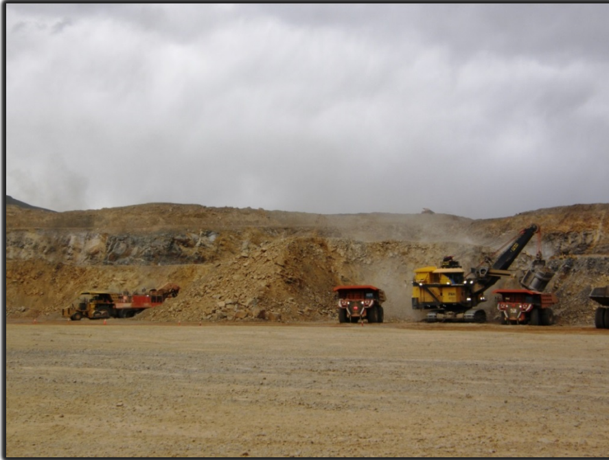
Mine shovels and trucks in the Mackay Pit at Marigold Mine. The diesel shovel is on the left and is approximately the same size as the haul trucks. The new electric shovel on the right towers over the haul trucks and can fill them with two buckets. A haul truck is dumping waste on the Northwest Waste Rock Storage Area in the background.
