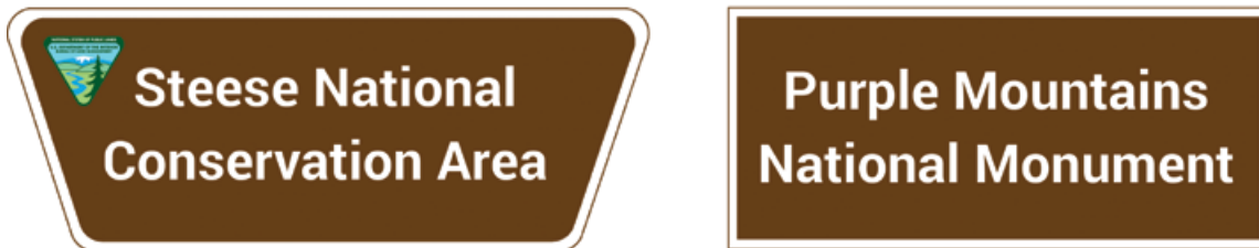
MUTCD-compliant identification signs.
