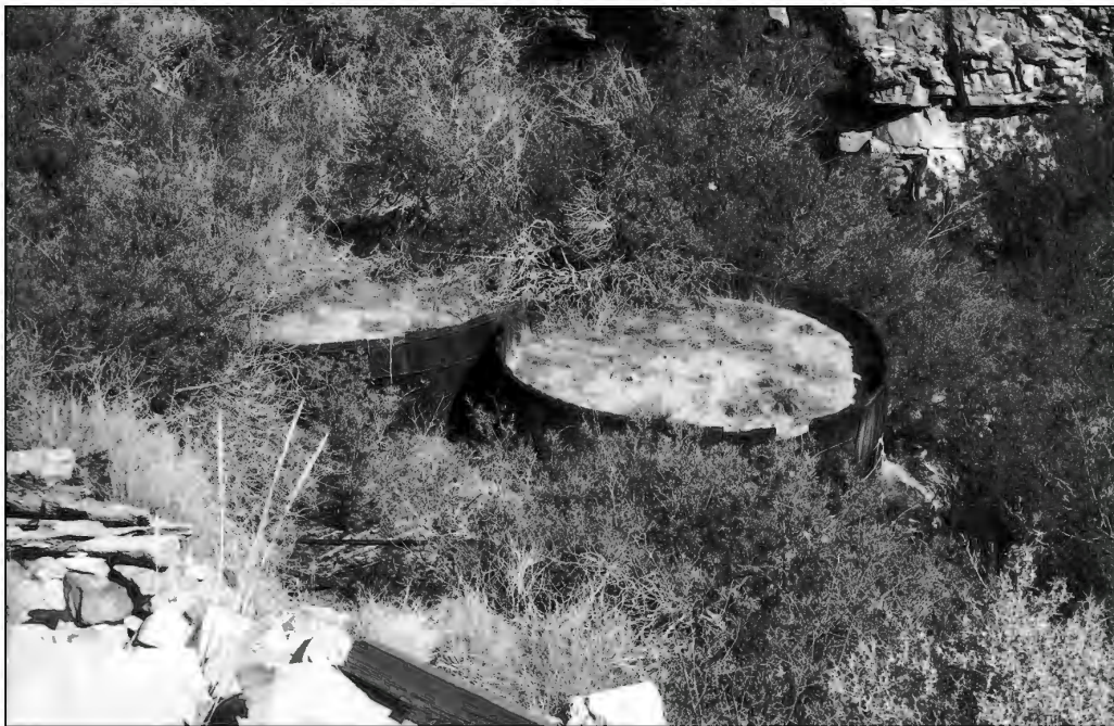
Figure 3.32. Redwood tanks containing mill tailings, Beveridge Mining District, 1991 (photograph by Karen K. Swope).
