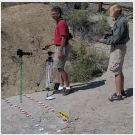
Figure A.s. It is important for the camera to maintain a consistent relation to the subject. Keeping a perpendicular angle to the subject is preferable. The dashed line represents the ray described in Appendix Figure A.4. A tripod with an extension arm was used when photographing a dinosaur trackway at the Red Gulch Dinosaur Tracksite, Wyoming.
