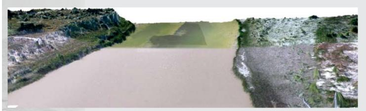
Figure 15. 3D image model developed from close-range photogrammetry along the Powder River, Wyoming. Images from two different times of year are merged to highlight the change in vegetation. With the 3D information available from multi-temporal 3D dataset, changes in vegetation heights, bank erosion, slope, water depth, vegetative cover, and bare ground can be measured (Noble et al. 2008).
