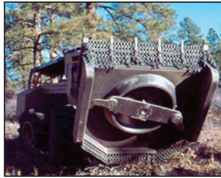
Figure 2. The Hydro-axe leaves behind a fine, protective mulch and causes little surface disturbance.
