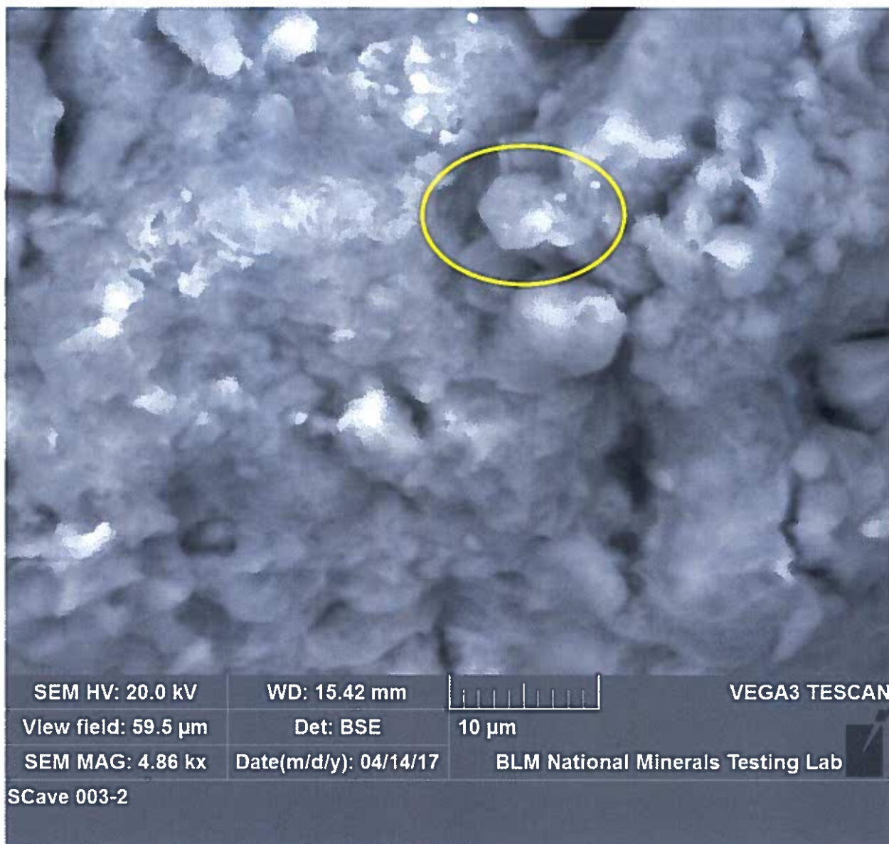
Image SCave 003-2: Magnification 4860X; a different perspective, note the clay particle (circled). No Erionite present.
