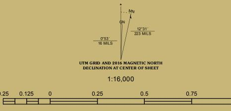
GPS coordinates (latitude and longitude) shown in degrees-minutes-seconds (D°M'S") format. Grid lines are shown in 1 - minute intervals. Grid ticks are shown in 10 - second intervals.
