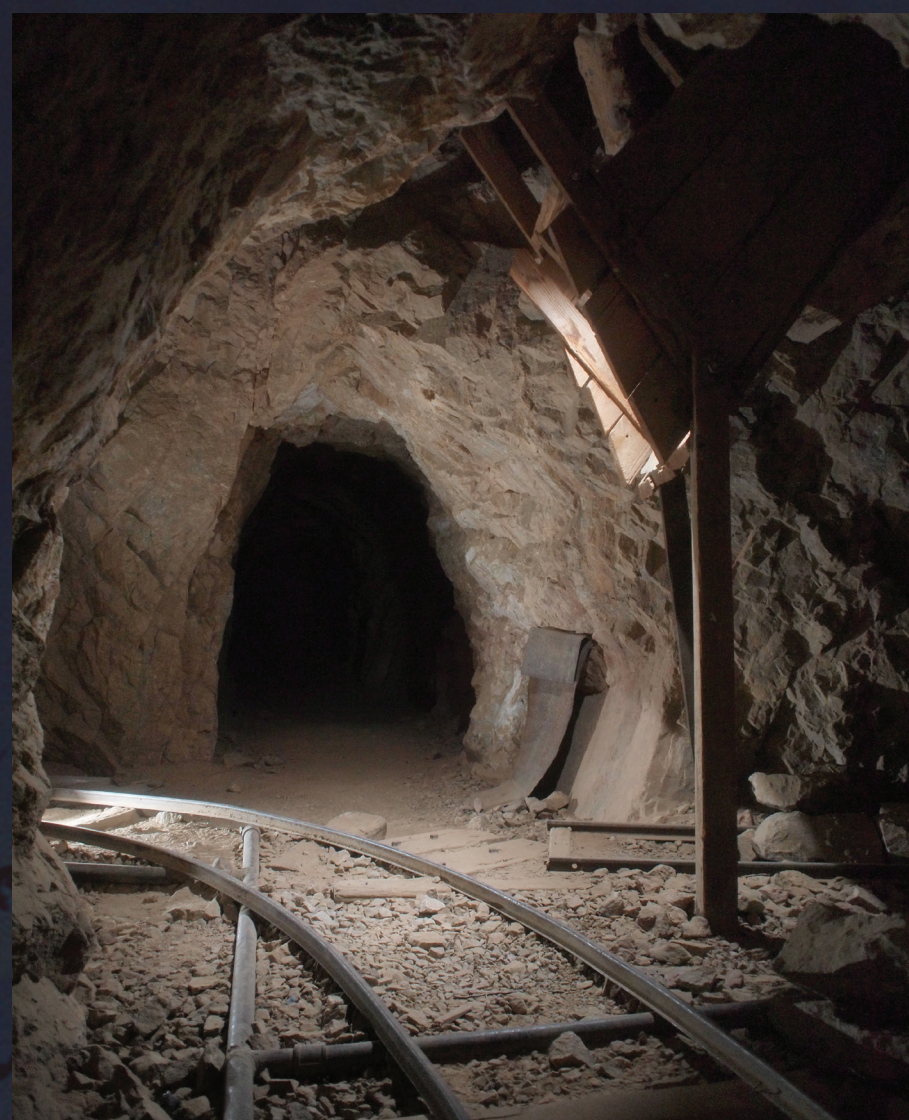
A drift in an abandoned mine, with an ore chute above ore cart rails.
