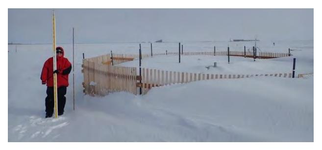
The Geonor precipitation gauge at Oliktok Point in April 2018, completely drifted over by the winter's heavy snow...but still sending out (erroneous) autonomous data.
