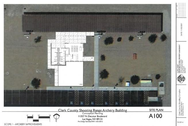
Figure 2 - New 3,000-SF Archery building with restrooms, a check-in area, and a storage/range management area
