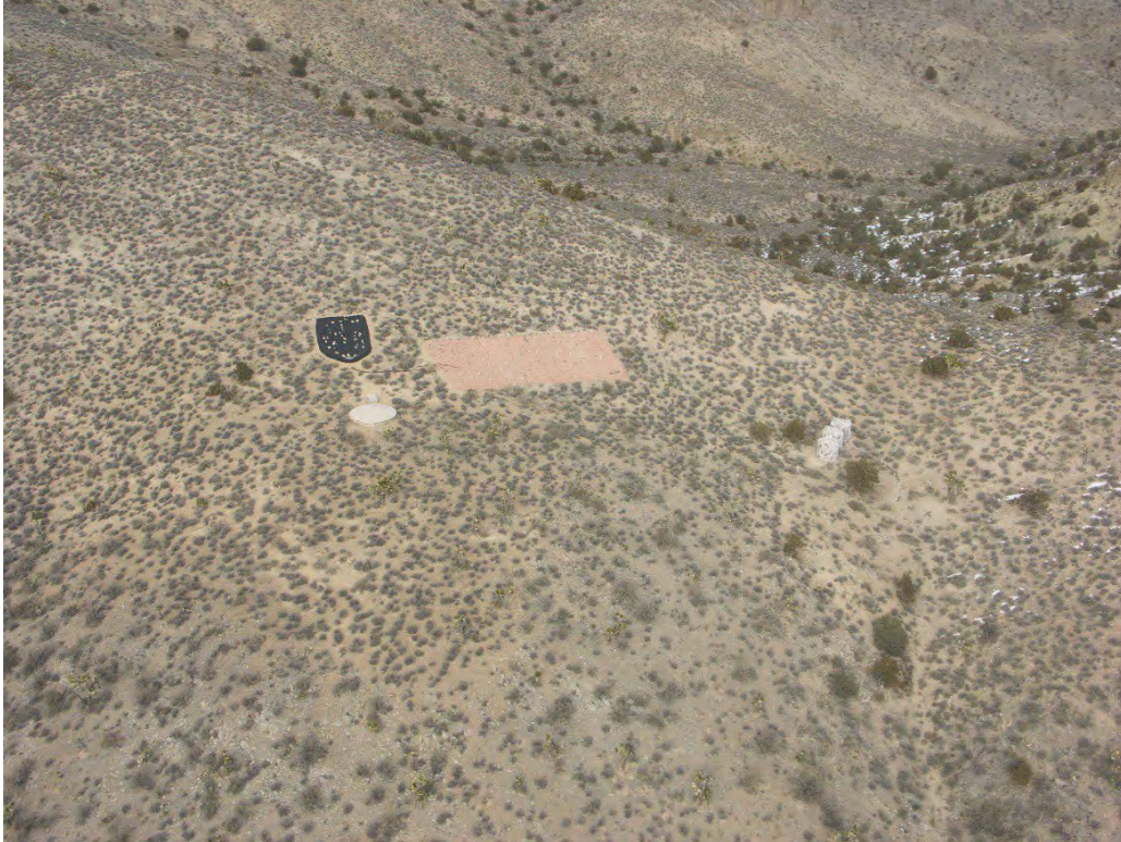
Figure 3. Overview of the Saddle Mountain project with older Hypalon aprons in the center and the 3upright tanks further to the right. The black apron and old circular storage tank are inoperable. This system will be replaced by a guzzler of updated design.
