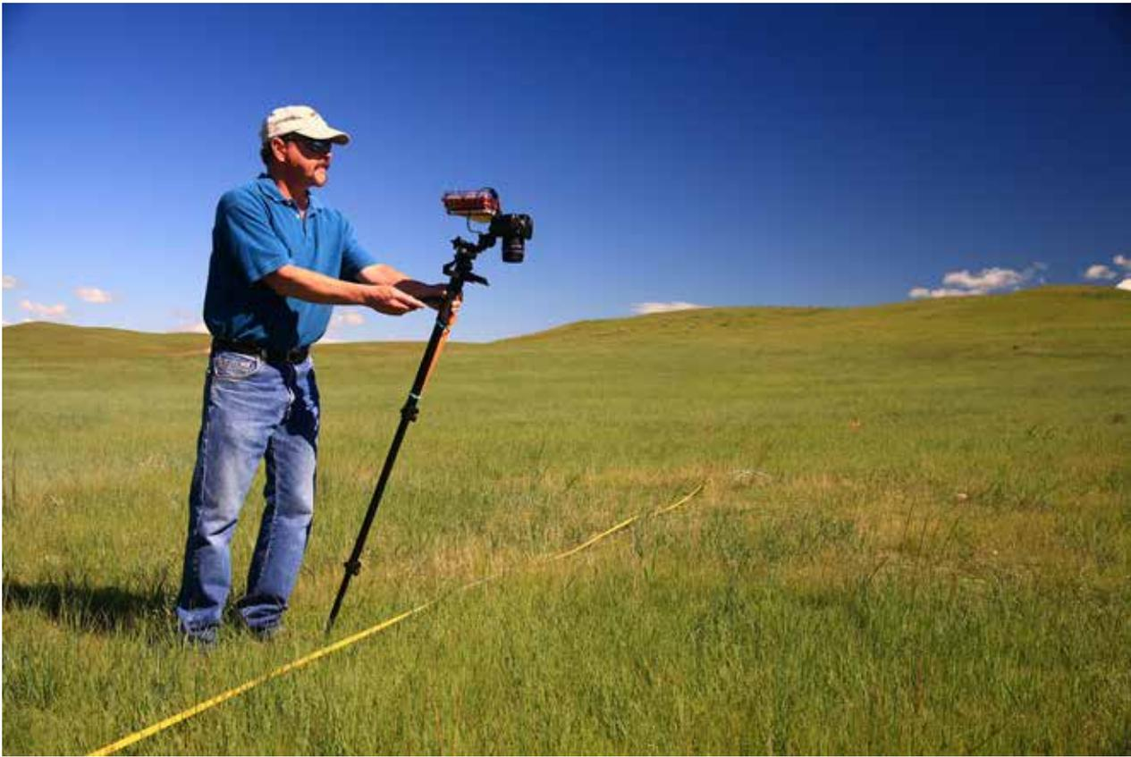
**Figure 9.** Example of proper image collection using an angled monopod placed at intervals along a field tape, with attention to operator shadow.
