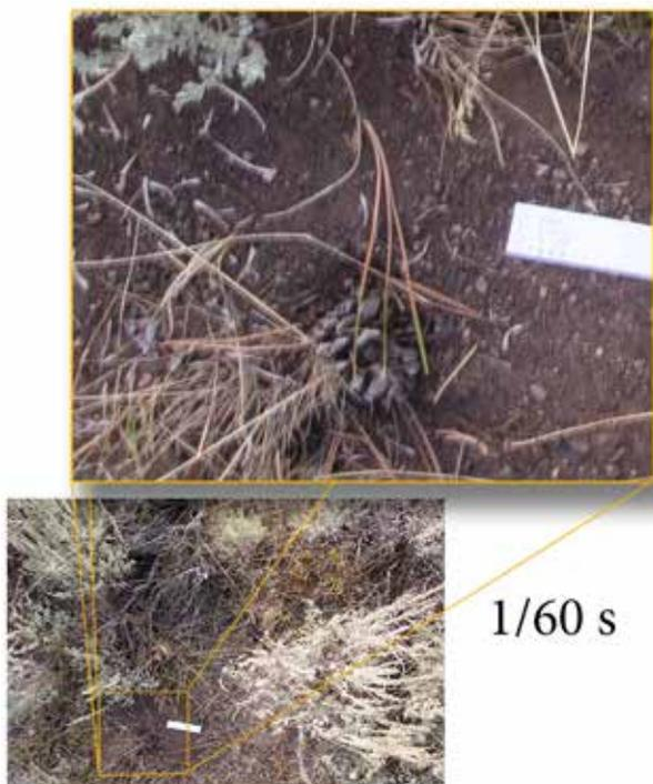
**Figure 8.** Always zoom in to 100% when reviewing images in the field. Images with slight motion blur can appear crisp and sharp at the small size of the camera display screen, illustrated by this marginal-quality image acquired with a shutter speed of 1/60 seconds. If noticed in the field, this plot could be rephotographed; this option is no longer available if the blur is not noticed until analysis commences weeks or months later.
