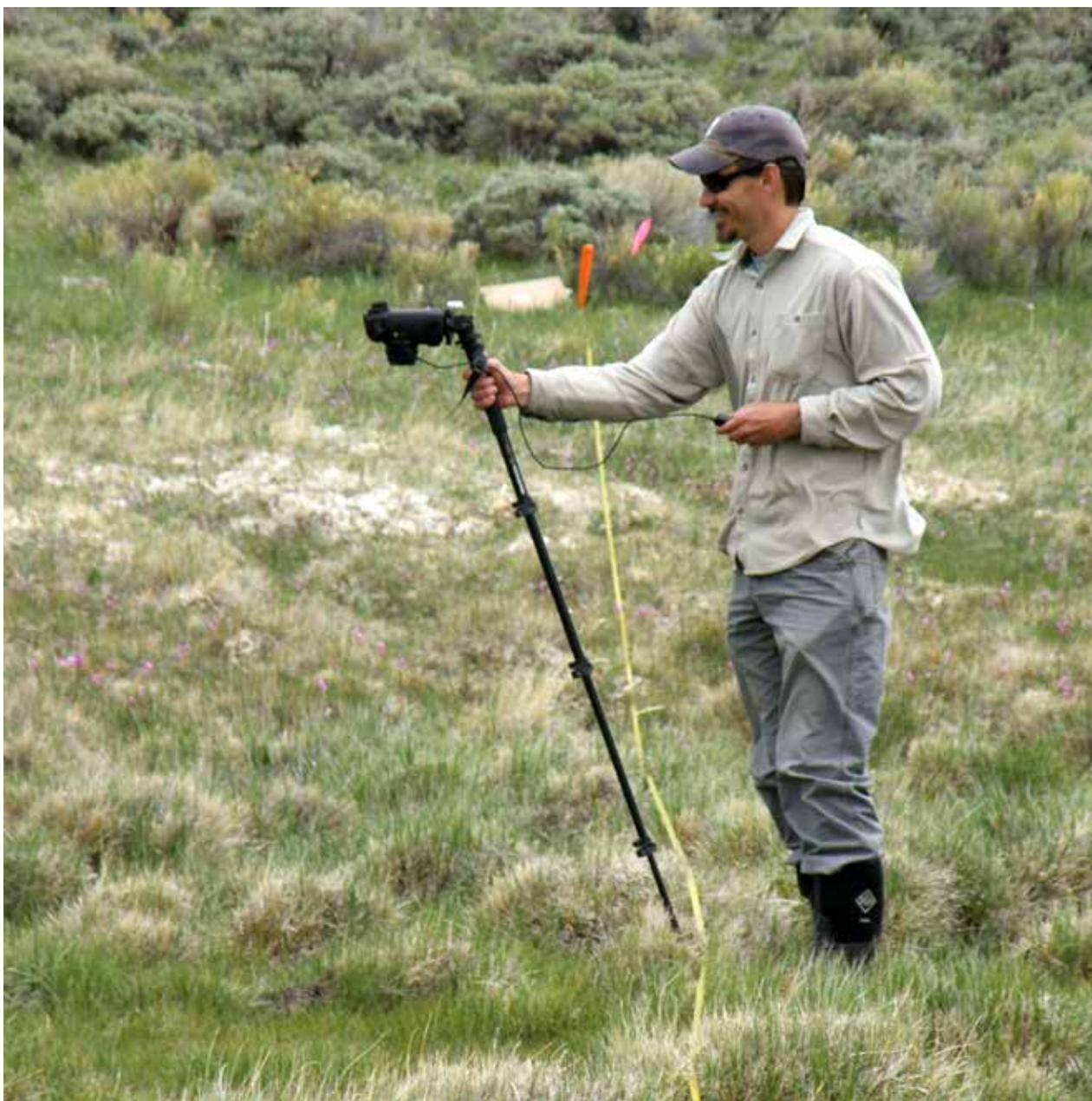
**Figure 1.** A camera in nadir position mounted on an angled monopod with no part of the monopod in the camera's field of view.
