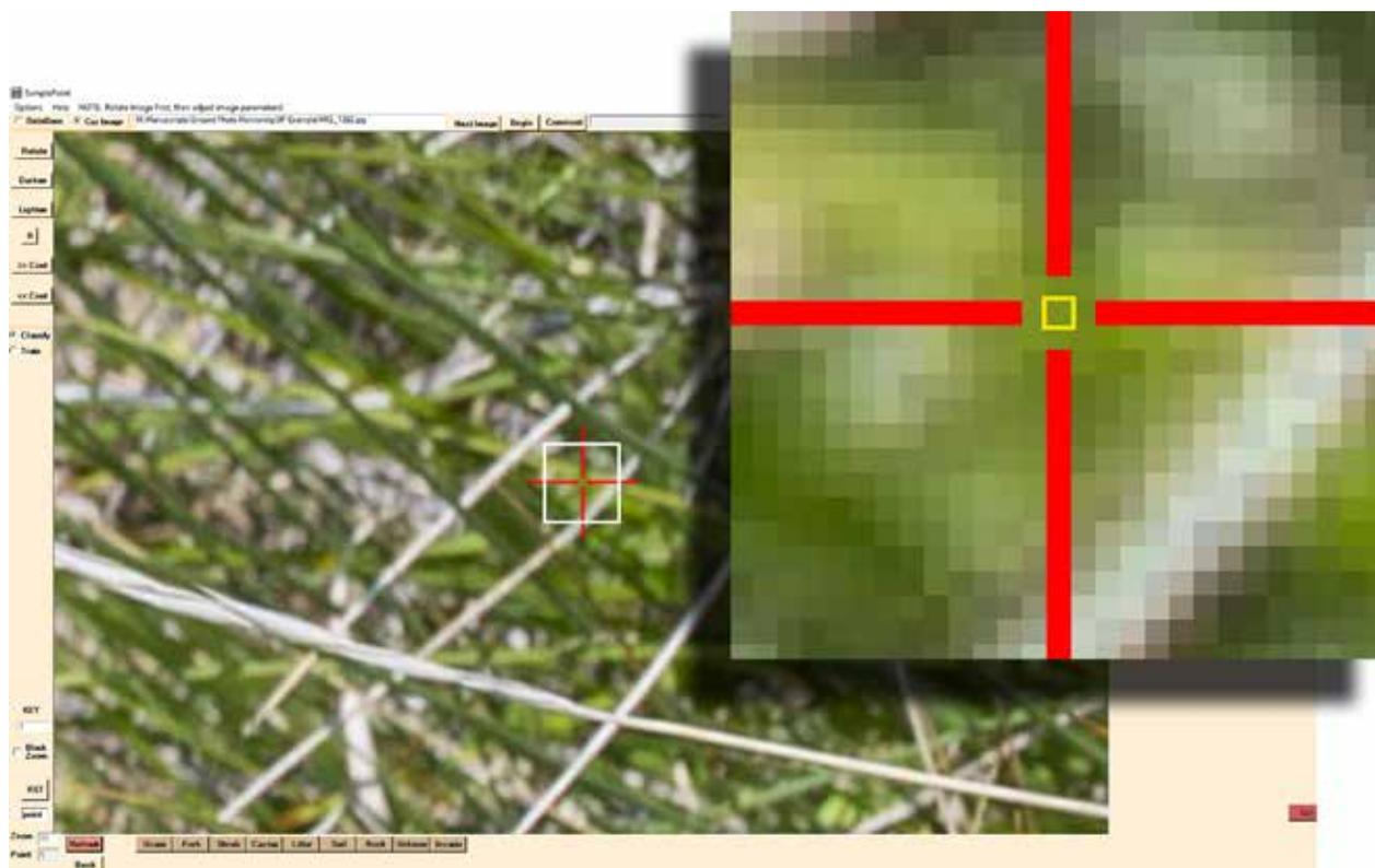
**Figure 12.** This SamplePoint screenshot shows the red classification crosshair. The white box outlines an area magnified in the inset, with the single pixel that should be classified highlighted in yellow here for illustration.
