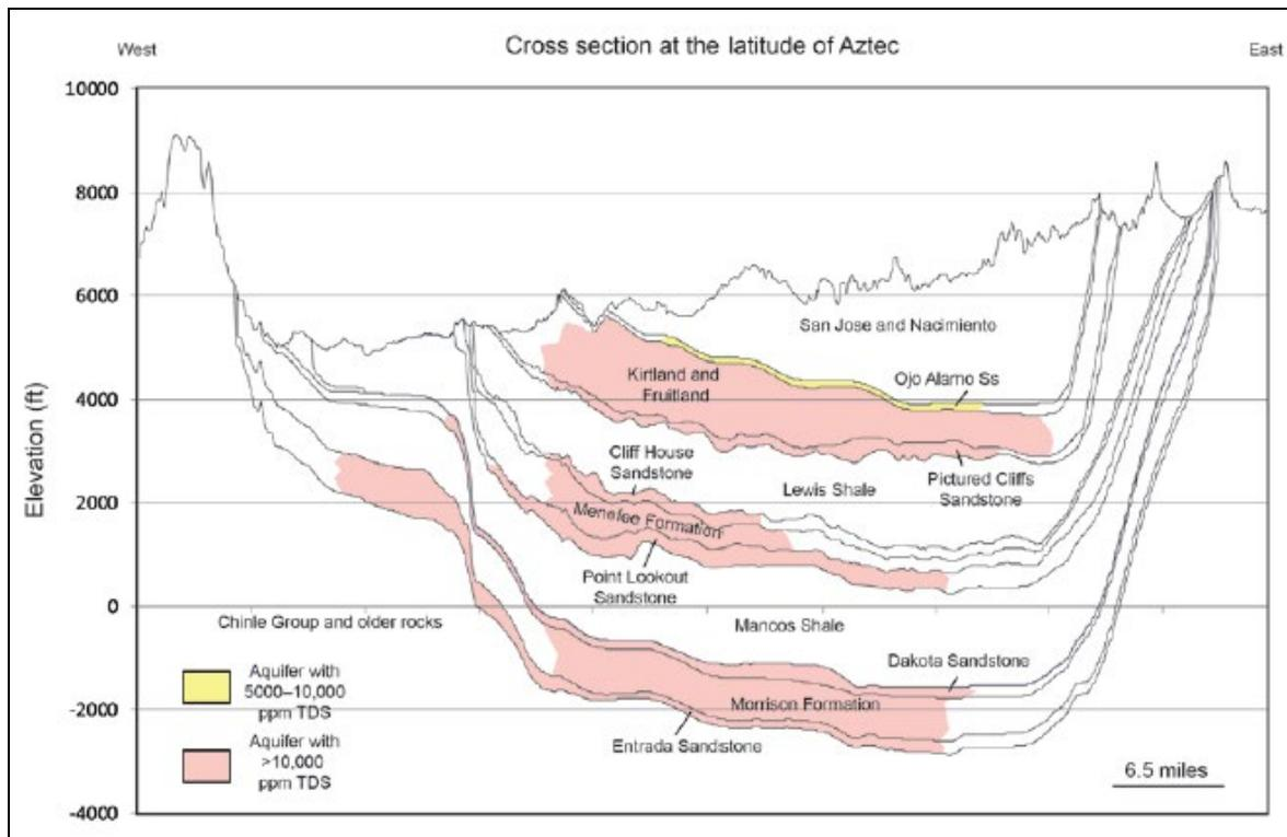
**Figure 5-2. Geologic cross section showing the distribution of saline aquifers in the San Juan Basin (Kelley et al., 2014).**
