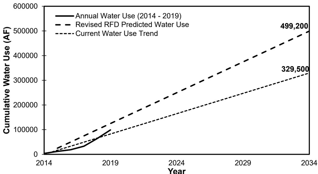
**Figure 3-2. Cumulative water use in the New Mexico Permian Basin (Chaves, Eddy, and Lea Counties) from 2014 to 2019 with projection to 2034. The revised Carlsbad RFD predicted usage of 31.2 AF/well or 24,960 AF/yr over a 20-year period. Current water use trend was derived from the average water use from 2014 to 2019 (26.8 AF/well or 16,474 AF/yr) projected to 2034. Cumulative water use data were collected from FracFocus (2020).**
