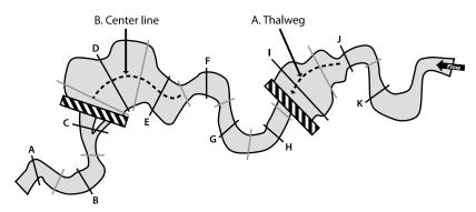
**Figure C2.** (**A**) Set up transects on a beaver-impacted stream following the flow of the thalweg if visible. (**B**) Set up transects perpendicular to the centerline of the beaver pool if the thalweg is not visible (Archer et al. 2015).
