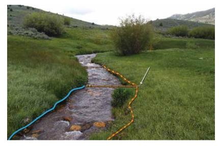
**Figure D9.** Location of scour line (blue line), bankfull, and bench heights. Bankfull and active bench heights are at the same elevation for this system (orange line). Note that the location of bankfull corresponds with the point at which the relatively flat bench begins to slope toward the water surface (white arrow). This is also shown by the depth rod, which is spanning the bankfull channel.
