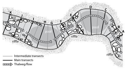
**Figure 1.** Typical reach setup with 11 main transects (A–K; black lines) and 10 intermediate transects (gray lines) oriented perpendicular to the thalweg. Reach lengths are equal to 20 x bankfull width or a minimum of 150 m.
