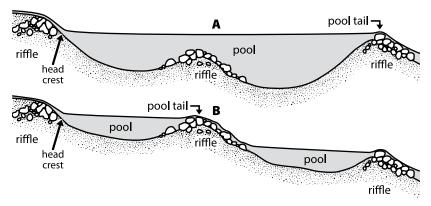
**Figure 21.** Examples of when two consecutive pools should be **(A)** lumped together because the pool is controlled by a single downstream pool tail that is shallower than the questionable upstream pool tail or **(B)** measured separately.
