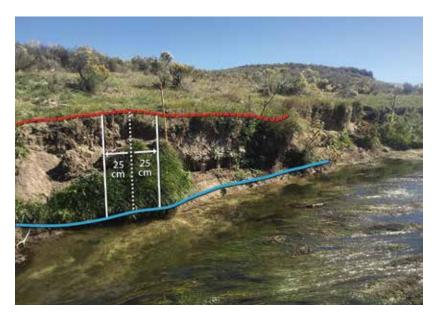
**Figure 13.** An erosional bank with a slump feature within the plot area (white lines). The slump counts as an erosional feature since it is located above scour line (blue line and plot lower limit). The upper plot limit is the bench (red line). This plot would be classified as covered and slump (S).
