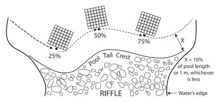
**Figure 22.** Locations and orientation of the pool tail fines grid relative to the pool tail crest (Saunders et al. 2019).
