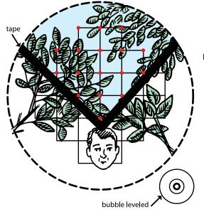
Figure 16. Modified densiometer. Count and record the number of grid intersection points within the V (0-17) that are covered by any form of vegetation or any object that creates shade, such as a canyon wall or bridge. In this example, the score would be recorded as 10 (USEPA 2009).
