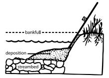
**Figure 28A.** Begin measuring the angle from the point where the deposition and bank meet (Archer et al. 2015).
