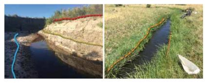
Figure 38. (A) Example of a critical concept photo with lines drawn on the photo to indicate scour line (blue), bankfull height (yellow), and bench height (red).(B) In this example, bankfull and bench heights are equal (orange).
