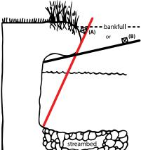
**Figure 31.** Bank angle is typically measured at the deepest point of a qualifying undercut (angle A). However, if the depth of the back of the undercut is consistent, measure bank angle at the highest elevation of the undercut (angle B), not angle A (Archer et al. 2015).
