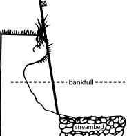
**Figure 32.** An undercut bank where the deepest point is elevationally above the ceiling of the undercut. These types of undercuts are recorded as 1° (Archer et al. 2015).
