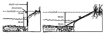
**Figure 34.** Measure the bank angle corresponding to the highest portion of the bank when the bank has two dominant angles (Archer et al. 2015).
