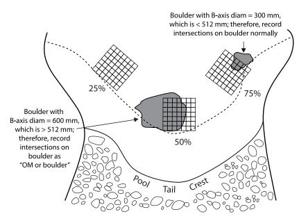
Figure 23. Rule set for measuring pool tail fines when the grid intersects boulders. Measurements should be taken for boulders < 512 mm and not for boulders ≥ 512 mm. For boulders ≥ 512 mm, record the number of intersections on the boulder as "OM (organic matter) or boulder" (PIBO 2019).
