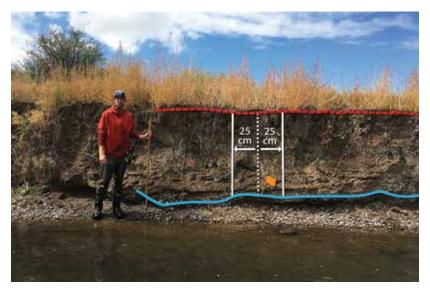
**Figure 15.** An erosional bank that is uncovered and eroding within the plot area (white lines). The blue line depicts the scour line (i.e., lower limit of the plot), and the red line depicts the first bench at or above bankfull (i.e., upper limit of the plot). The bank is within 10 degrees of vertical and is < 50% covered; therefore, it would be classified as uncovered and eroding (E).
