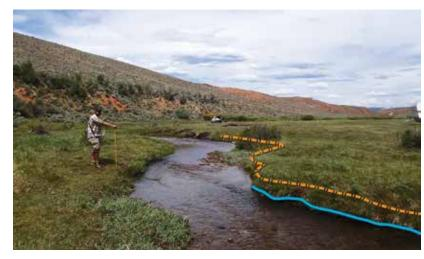
**Figure D1.** Location of scour line (blue line), bankfull, and bench heights. Bankfull and active bench heights are at the same elevation for this system (orange line). This system has a broad valley bottom and is well connected to an active bench that is frequently inundated during bankfull flows.
