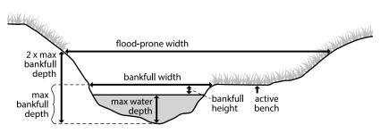
**Figure 25.** Locations of the three measurements critical to determining floodprone width: maximum water depth, bankfull height, and bankfull width (Harman et al. 2012). Note that if the flood-prone width is > 3 times the bankfull width, stop measuring and record that value.
