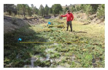
**Figure D10.** Example of a low energy system where identifiable bankfull features are not present at every transect. Transect E does not have identifiable bankfull or scour line features and should not be sampled as the protocol cannot be appropriately applied. Reach point coordinates should be moved to ensure that 5 or more transects have identifiable bankfull features.
