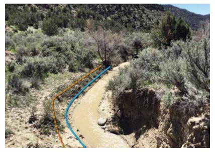
**Figure D4.** Location of scour line (blue line), bankfull, and bench heights. Bankfull and active bench heights are at the same elevation (orange line). Scour line is indicated by the lower extent of sod-forming vegetation and the indentation in the bank.
