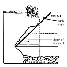
Figure 30. Measure undercut bank angle from the deepest point to the ceiling of the undercut; determine if the undercut has a qualifying depth (≥ 5 cm) by lowering the depth rod until it is horizontal (Archer et al. 2015).
