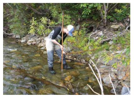
**Figure 4.** Example of how to use two depth rods to measure bankfull or bench height. For this transect, bankfull and bench height are at the same elevation. Note the position of the horizontal depth rod, which is at the same elevation of the flat, bench surface.
