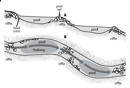
**Figure 19. (A)** Cross-sectional view and **(B)** bird's eye view of a pool, showing pool features. Pools are identified by the concave shape bound by a head crest and tail and a max depth > 1.5 times the pool tail depth (modified from Dunne and Leopold 1978).
