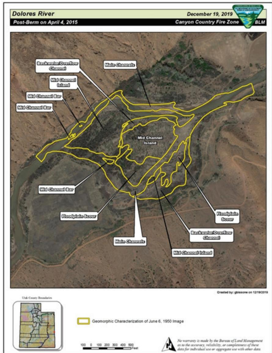
Figure 3. Post-Berm River in 2015 with pre-berm features overlain.
