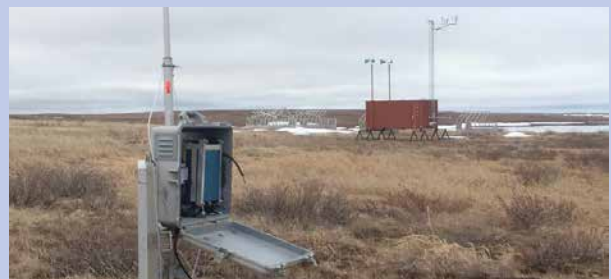
Portable ozone monitor with a high-quality particle size distribution meteorological station in the background.
