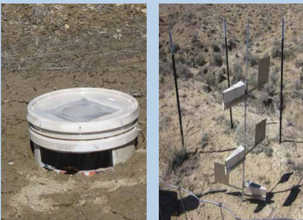
Dust and wind erosion monitoring equipment in the Badger Wash in western Colorado.
