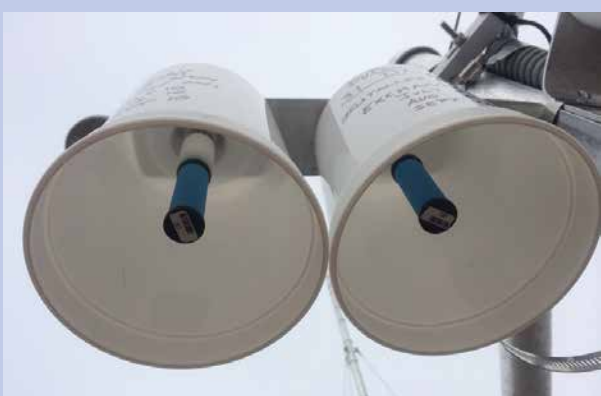
Passive ammonia samplers installed at the Inigok field camp in the National Petroleum Reserve in Alaska.
