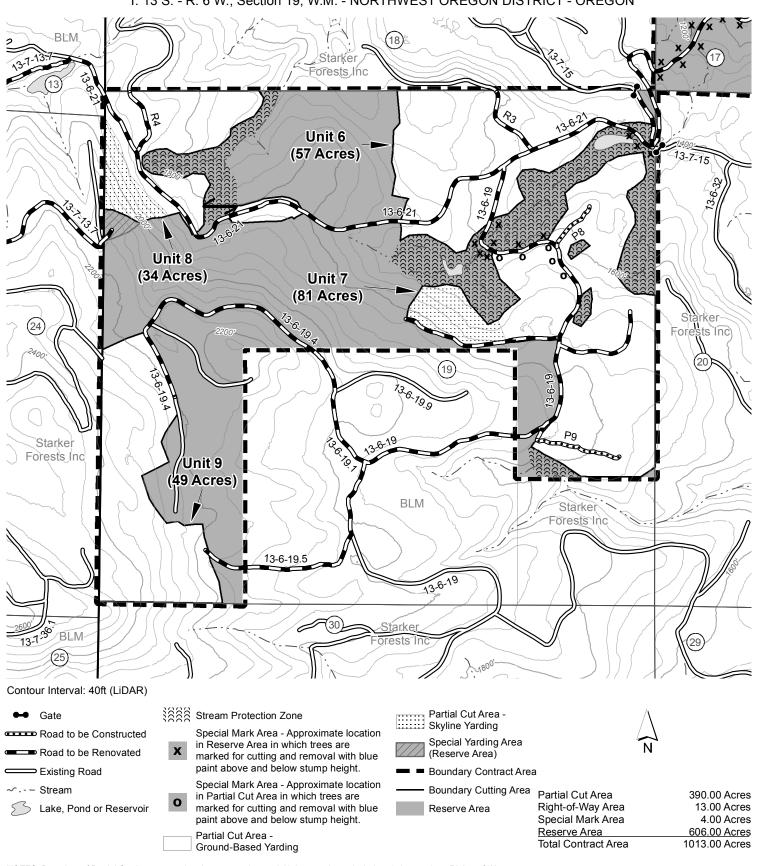
NOTES: Boundary of Partial Cut Areas are painted orange and posted. Unit acres do not include existing roads or Rights-of-Way. Acres shown on Exhibit A have been computed using a Trimble Geo XT Global Positioning System receiver. Acreage was calculated based on Global Positioning System traverse procedures including differential correction.
