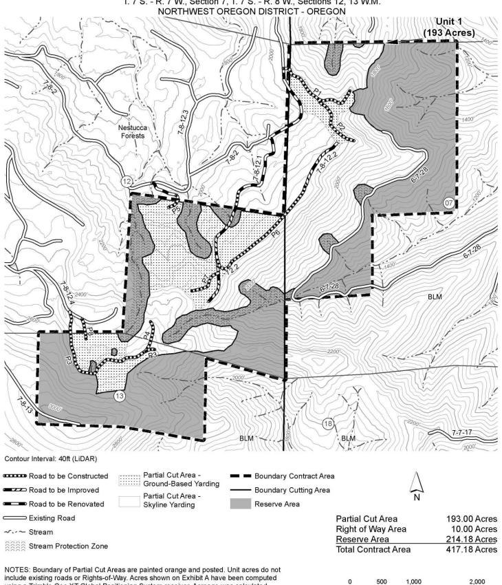
include existing roads or Rights-of-Way. Acres shown on Exhibit A have been computed using a Trimble Geo XT Global Positioning System receiver. Acreage was calculated based on Global Positioning System traverse procedures including differential correction. Form 5450-3a (February 1986)
