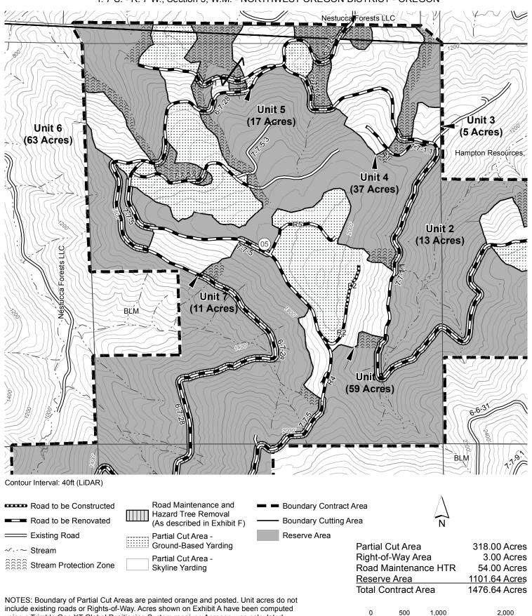
include existing roads or Rights-of-Way. Acres shown on Exhibit A have been computed using a Trimble Geo XT Global Positioning System receiver. Acreage was calculated based on Global Positioning System traverse procedures including differential correction.
