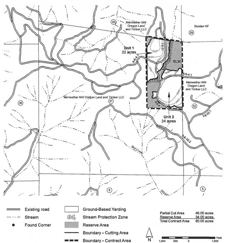
NOTES: Boundary of partial cut areas are painted orange and posted. Unit acres do not include existing roads. Acres shown on Exhibit A have been computed using a Trimble Geo XT Global Positioning System Receiver. Acreage was calculated based on Global Positioning System traverse procedures including differential correction.
