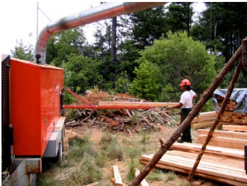
The Economizer, a small portable log mill converts small diameter logs into lumber.
