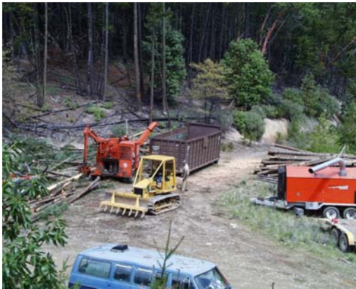
On site chipping operation converting tops and limbs into 'hog fuel' for use at Biomass One.
