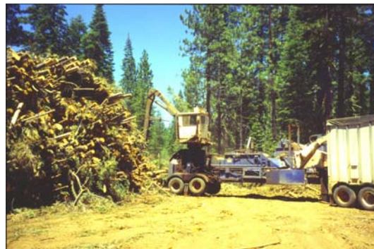
Chipping non-merchantable material from a timber sale directly into trucks.
