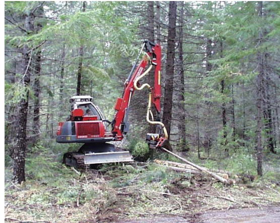
A small diameter harvest operation uses a “dangle head processor” to remove small diameter trees.
