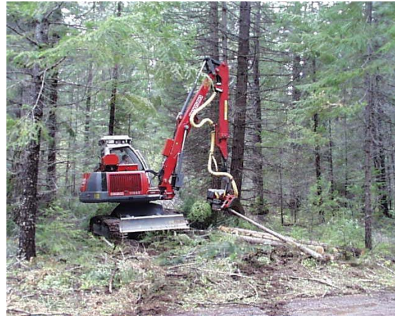
A small diameter harvest operation uses a “dangle head processor” to remove small diameter trees.
