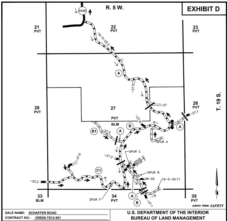
LEGEND **\_\_\_\_ BLM MAINTAINED ROADS PURCHASER MAINTAINED ROADS**  $\Lambda$ **PAVED ROAD ROCKED ROAD NATURAL SURFACE ROAD TIMBER HAUL ROUTE** MINERAL HAUL ROUTE **SEGMENT BREAK ROAD SEGMENT STOCKPILE** GATE
