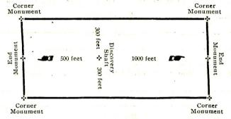
The above diagram is to give the locator a general idea of the plan of location under new law. Your discovery shaft may be in the center of
