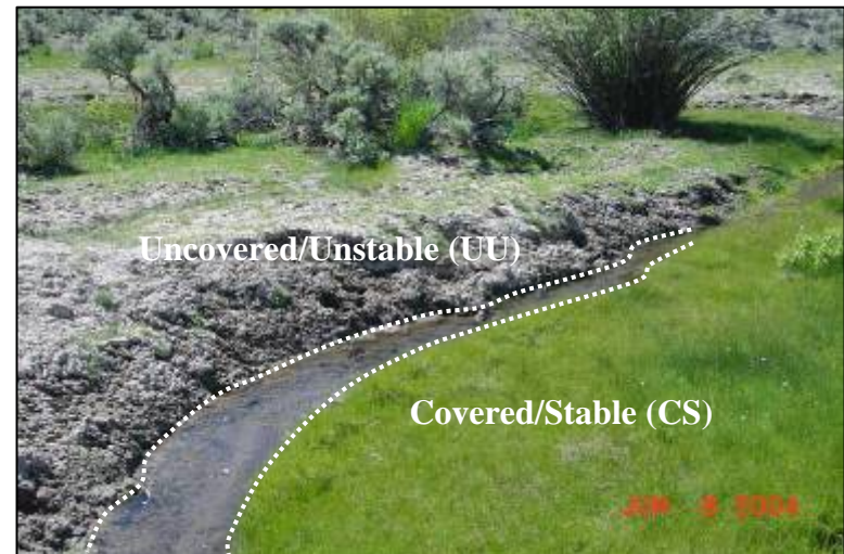
Figure 11 —the streambank on one side of the stream is uncovered/unstable (UU) and the other side is covered/stable (CS).
