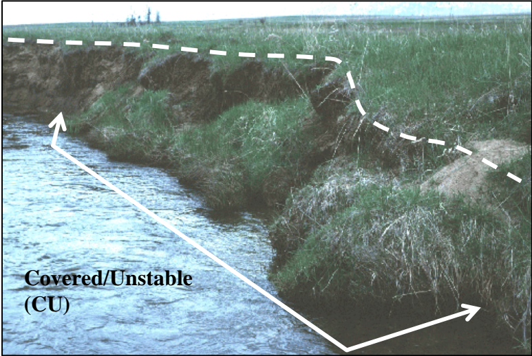
Figure 9 —slump blocks and slumping banks with the blocks and attached bank above the scour line are covered/unstable (CU).
