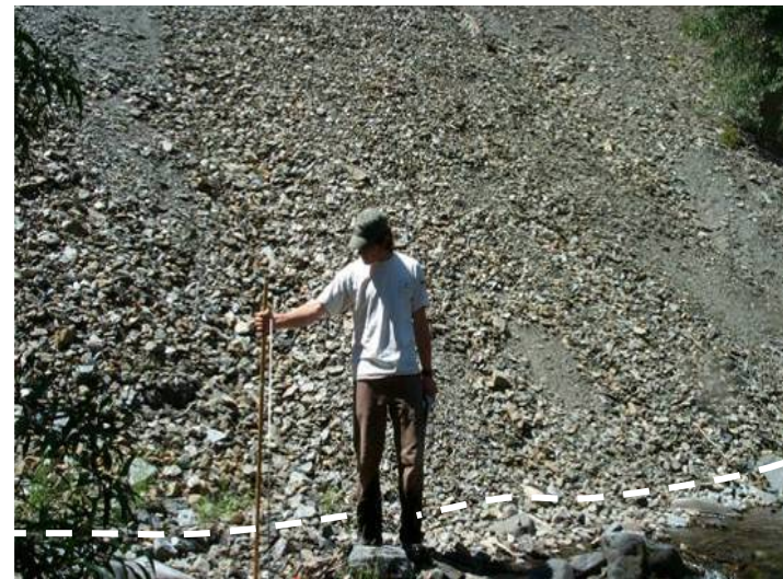
Figure 25 —the greenline along talus slope is considered as rock and is at about the bankfull stream level. Record the data as rock. Photo - PIBO, U.S. Forest Service
