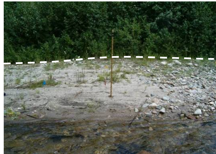
Figure 8 —greenline follows the relatively continuous line of vegetation and not the scatter vegetation on the sand/gravel bar. Photo - PIBO, U.S. Forest Service
