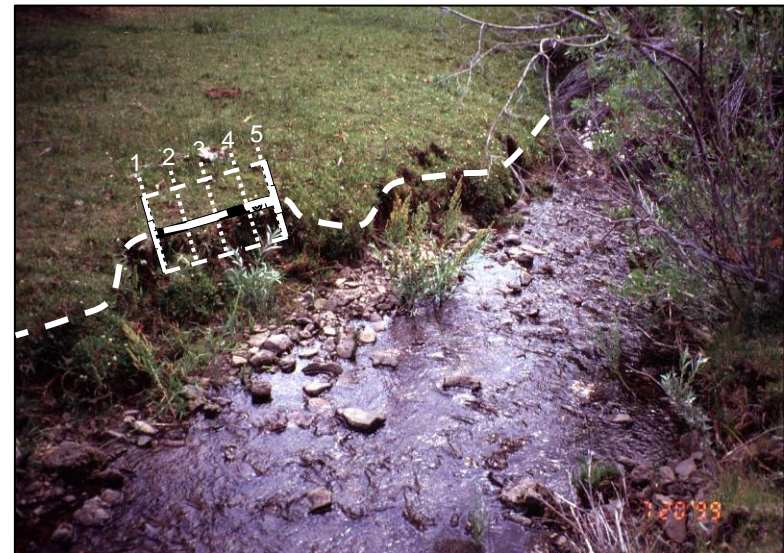
Figure 2 —the monitoring frame is centered on the greenline and the number of lines (0 to 5) that intersect streambank alteration (trampling or shearing) is counted and recorded. Lines 1, 2, 4, and 5 intersect streambank alteration. Four is recorded.
