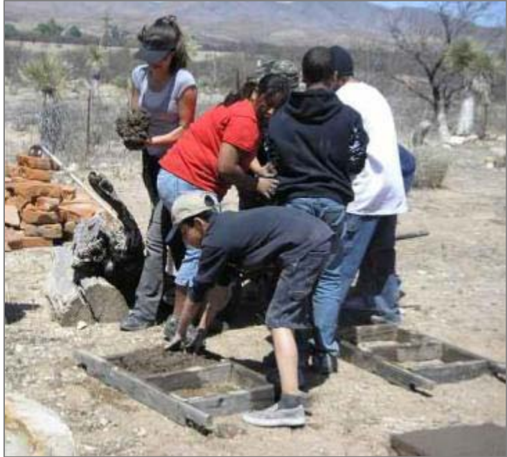
Figure 16- Hohokam Middle School students of the Pascua Yaqui Nation make adobe bricks at LCNCA as part of the Youth in Wilderness Program
